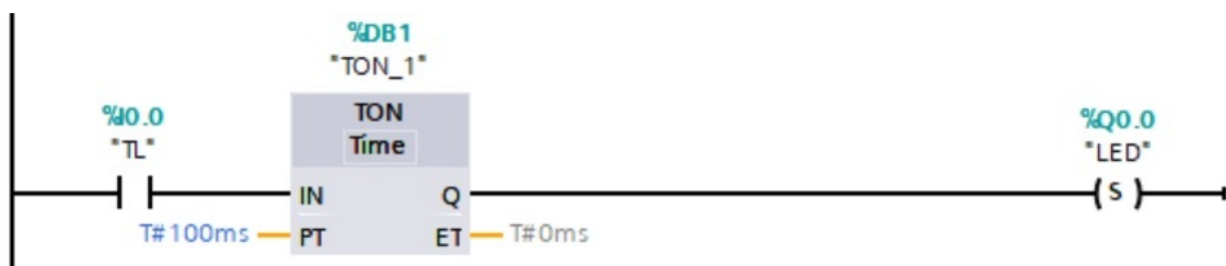
Obr. 4.183. Program v OB30 pre zapnutie LED
